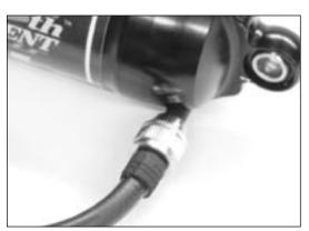
as a result of a worn pump fitting o-ring that needs replacement. Do not ride the bike until the shock is properly pressurized.
