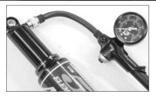
2. Installing Air Pressure – Remove the air cap from the Schrader valve on the end of the shock body. Attach the pump to the Schrader valve. Some people damage their pumps by screwing them on too far. As soon as the gauge registers pressure, screw 1/2 turn more and pump to the desired level. Use the release button on
