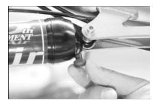
When reaching the minimum & maximum stops of the adjuster range, do not apply excessive force to continue turning the adjuster, or damage to the adjuster will occur that is not covered by the warranty.
