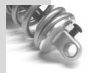
For models fitted with the inset 4mm hex allen knob, you can use the same ball driver or allen wrench used to adjust the beginning & ending stroke adjusters. When using the 4mm ball driver, adjustment only requires a **light force** to turn the adjuster. Turning the knob clockwise will increase (slow down) the rebound damping & turning the knob counterclockwise will decrease (speed up) the rebound damping.
