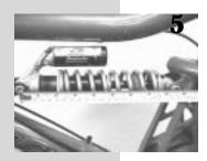
Element shock works best with slightly more sag than conventional shocks. The recommended amount of sag is 30-40% for downhill, 30-40% for free-ride and 25-35% for cross-country. Never exceed 8mm/.325" preload of the spring.
