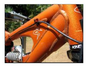
The seat-tube / top tube junction has also received some serious attention. The 'free utilises a dropped top-tube for increased standover clearance with a big, don't argue piece of bracing connecting the top and seat-tubes to still give a full 17.5" seat-tube length on our medium sized frame.
